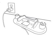
2. The LED lights on the front will briefly flash to indicate that it's connected properly. If AA NiMH rechargeable batteries are inserted, the LED lights will turn RED which indicates charging. The power source is charging both your headset and the rechargeable batteries simultaneously.
